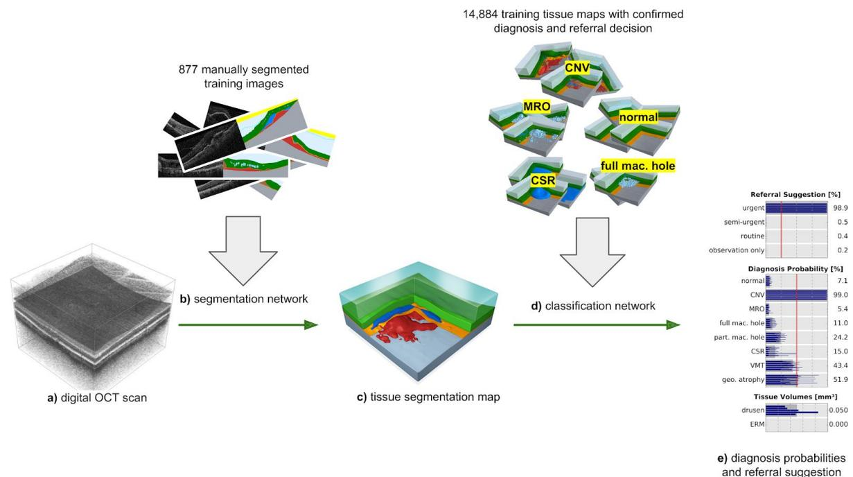
**Figure 1 | Our proposed AI framework.** (a) Raw retinal OCT scan ( $6 \times 6 \times 2.3 \text{ mm}^3$  around the macula). (b) Deep segmentation network, trained with manually segmented OCT scans. (c) Resulting tissue segmentation map. (d) Deep classification network, trained with tissue maps with confirmed diagnoses and optimal referral decisions. (e) Predicted diagnosis probabilities and referral suggestions.
