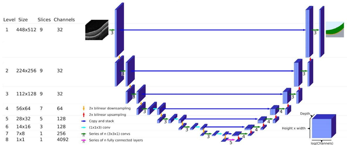
**Supplementary Figure 14 | 3D U-Net model used in the first stage of our approach.** At training time, the model receives 9 contiguous OCT slices. Blue boxes illustrate the 4D activation maps. Colored arrows stand for the different operations.
