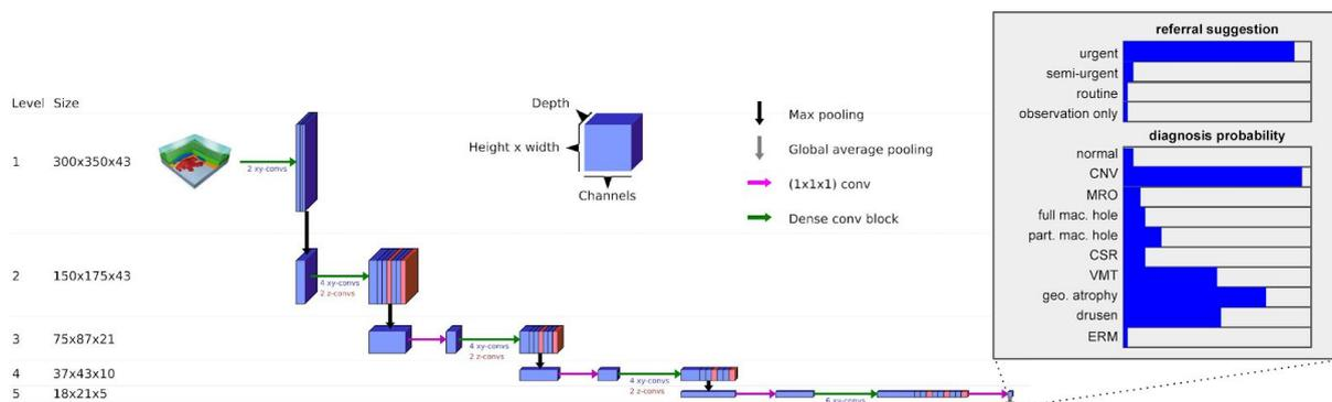
**Supplementary Figure 16 | Classification CNN (convolutional neural network) used in the second stage of our approach.** Blue and red boxes illustrate the 4D activation maps. Blue boxes are the result of a (3x3x1) convolution, while red boxes are the result of a (1x1x3) convolution.
